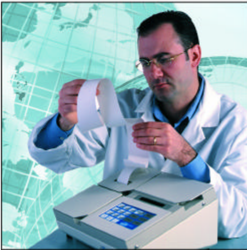
Gentleman using a fluorometer to read mold count results from VICAM's MoldQuant-T test, a quantitative test for tomato mold.
